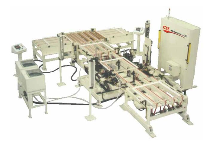
The **CSE Automation, LLC Automatic Sash Clamp** is built for high production. This machine can economically change size for each cycle of the machine. Production capacity is approximately 1,000 to 1,500 sashes per eight-hour shift.
