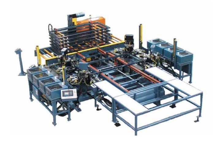
The CSE Automation, LLC Premier Automatic Storm Door Machine is designed to automatically clamp and fasten aluminum storm doors. This machine is capable of producing 1,200 to 1,500 per eight hour shift.
