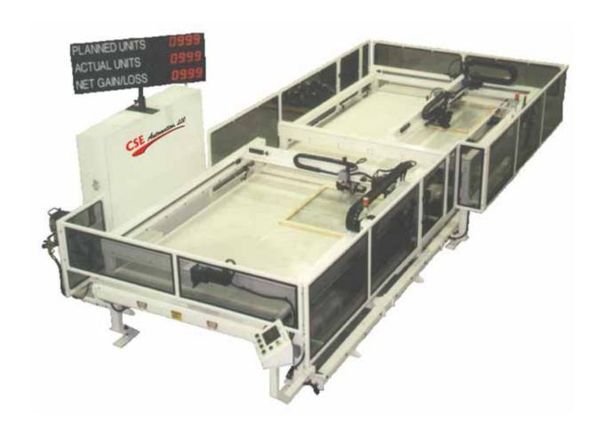
The CSE Automation, LLC Premier Bead Nailer is is designed to automatically fasten glazing stops to window sash or patio doors. This machine is capable of producing 1,200 to 1,500 sashes per shift.
