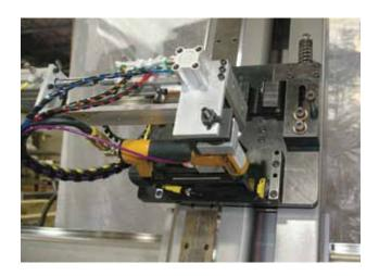
Adjustable clamp pads to accommodate 1-1/4" to 3-1/2" stile sizes at 1/8th" increments
