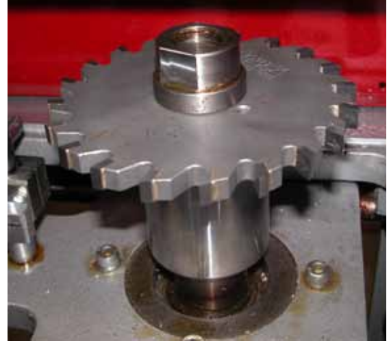
▲ Example of custom cutter installed
