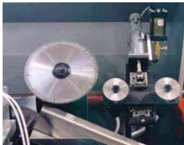
Internal view of Expanded Capacity Frame Notching Saw with auxiliary 45° finish notch assembly
