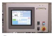
Operator interface via industrial grade PC workstation with flat panel liquid crystal color display, touch screen functionality and Windows-based operating system. Features:
