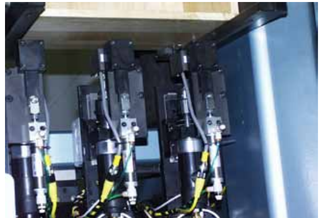
Drawer front multi-position center and corner drilling.
