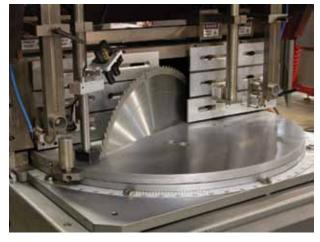
Up to 600 mm (23.6") diameter, bottom-feed blade and large tabletop work surface allow for accurate cutting of miter angles from 15° inside to 90° to 15° outside
