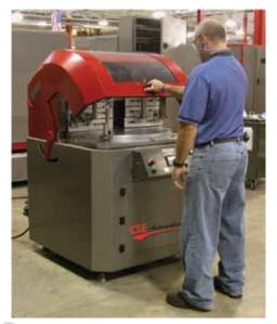
Enclosed hood guard offers protection to operator from flying debris and sawblade
