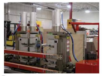
Machine design features rear approaching heat plates with easy access for maintenance and Teflon paper change-over.
